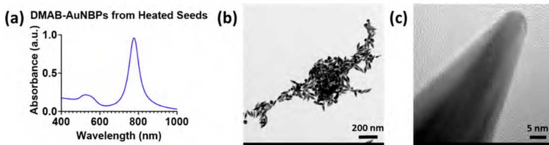
Figure 6. Characterization of AuNBPs synthesized using heated seeds. (a) UV-vis spectrum of synthesized NBPs from heated Au seeds. (b,c) FEG-TEM (300 keV) images of NBPs synthesized using citric acid-containing seeds.
